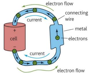
The size of the current is measured in **Amperes** using an ammeter. The faster the electrons move the larger the current.
